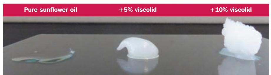
**Figure 3:** Pure Sunflower oil and after thickening with dermofeel viscolid.
